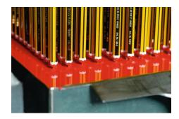
During production, Noris 120 pencils receive their characteristic coloured cap at the end of the pencil, which has shown the hardness of the lead since 1955.
